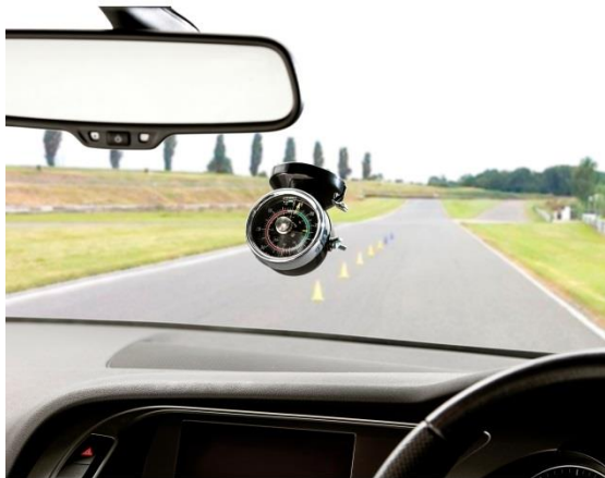
Brakemeter mounted to windscreen using its built-in suction cup.
