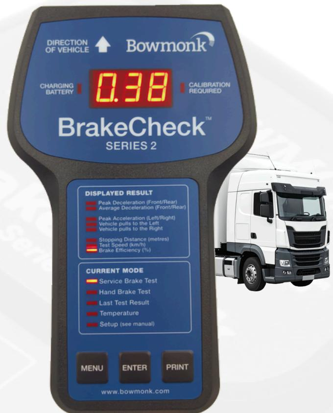
Designed to be self-compensating, the instrument will indicate on the LED screen when it is positioned level enough to perform a brake test, with a generous tolerance to ensure that this is easy to achieve.
